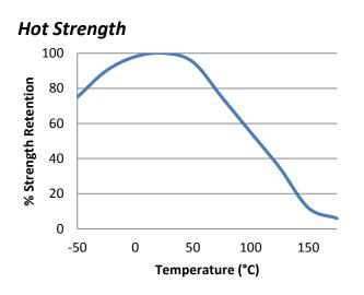
"Hot strength" shear strength tests performed on mild steel. 24hr cure at room temperature and conditioned to pull temperature for 30 minutes before testing.
