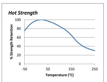
"Hot strength" shear strength tests performed on mild steel. Initially cured at room temperature and then post-cured at 150°C for 2 hours. Test pieces conditioned to pull temperature for 30 minutes before testing.
