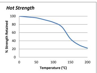
"Hot strength" shear strength tests performed on mild steel. Fully cured then conditioned to pull temperature for 30 minutes before testing. ES5562 can withstand higher temperatures for brief periods (such as for paint baking and wave soldering processes) providing the joint is not unduly stressed. The minimum temperature the cured adhesive can be exposed to is -40°C (-40°F) depending on the materials being bonded.
