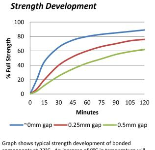
Graph shows typical strength development of bonded components at 23°C. An increase of 8°C in temperature will halve the cure time. Lower temperatures will result in a slower cure time.
