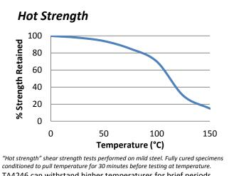
conditioned to pull temperature for 30 minutes before testing at temperature. TA4246 can withstand higher temperatures for brief periods (such as for paint baking and wave soldering processes) providing the joint is not unduly stressed. The minimum temperature the cured adhesive can be exposed to is -40°C (-40°F) depending on the materials being bonded.
