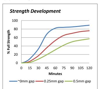
Graph shows typical strength development of bonded components at 23°C. An increase of 8°C in temperature will halve the cure time. Lower temperatures will result in a slower cure time.
