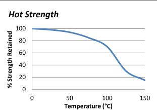
"Hot strength" shear strength tests performed on mild steel. Fully cured specimens conditioned to pull temperature for 30 minutes before testing at temperature. TA435 can withstand higher temperatures for brief periods (such as for paint baking and wave soldering processes) providing the joint is not unduly stressed. The minimum temperature the cured adhesive can be exposed to is -55°C (-65°F) depending on the materials being bonded.
