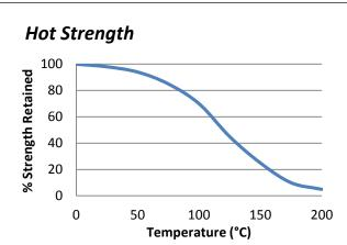
"Hot strength" shear strength tests performed on mild steel. Fully cured specimens conditioned to pull temperature for 30 minutes before testing at temperature. TA436 can withstand higher temperatures for brief periods (such as for paint baking and wave soldering processes) providing the joint is not unduly stressed. The minimum temperature the cured adhesive can be exposed to is -55°C (-65°F) depending on the materials being bonded.
