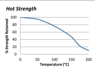
"Hot strength" shear strength tests performed on mild steel. Fully cured specimens conditioned to pull temperature for 30 minutes before testing at temperature. TA439 can withstand higher temperatures for brief periods (such as for paint baking and wave soldering processes) providing the joint is not unduly stressed. The minimum temperature the cured adhesive can be exposed to is -55°C (-65°F) depending on the materials being bonded.
