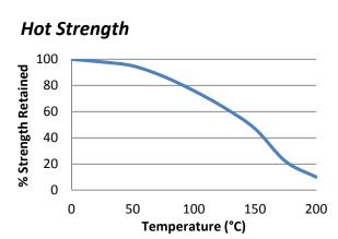
"Hot strength" shear strength tests performed on mild steel. Fully cured specimens conditioned to pull temperature for 30 minutes before testing at temperature. TA459 can withstand higher temperatures for brief periods (such as for paint baking and wave soldering processes) providing the joint is not unduly stressed. The minimum temperature the cured adhesive can be exposed to is -55°C (-65°F) depending on the materials being bonded.
