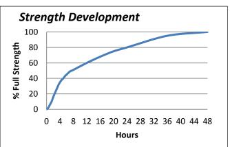
Graph shows typical strength development of bonded components at  $23^{\circ}$ C. An increase of  $8^{\circ}$ C in temperature will halve the cure time. Lower temperatures will result in a slower cure time.
