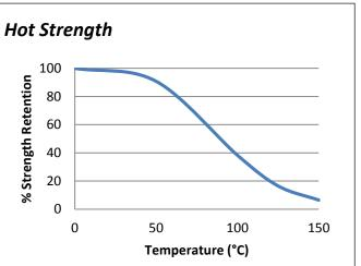
TA4810 can withstand higher temperatures for brief periods (such as for paint baking and wave soldering processes) providing the joint is not unduly stressed. The minimum temperature the cured adhesive can be exposed to is -40°C (-40°F) depending on the materials being bonded.
