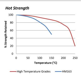
"Hot strength" shear strength tests performed on mild steel. 24hr cure at room temperature and conditioned to pull temperature for 30 minutes before testing.
